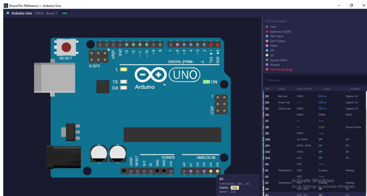
Board View — Board Pin Reference for a connected Arduino Uno, pins colour-coded by current function
